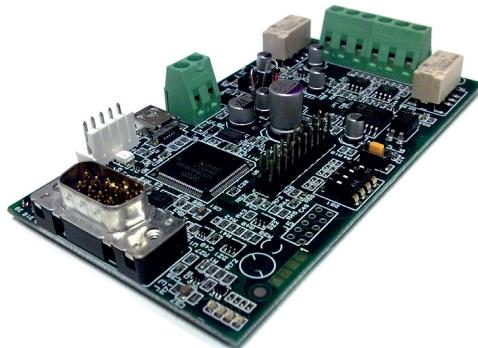
Expansion card for Toccare® fire control panel. It allows to connect up to 64 control panels in a ring network, allowing to share information and set crossed output activation.
