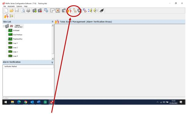
Select the False Alarm Management icon, under alarm Verification the method is not selected.
