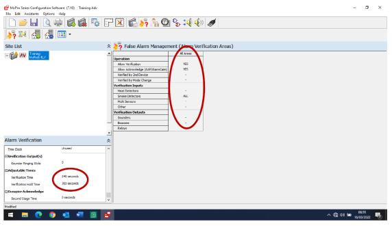
Select type 'B' method – the verification time will be defaulted to 240 seconds and all the smoke detectors are added by default.
