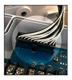
Connect the head to the base plate by first plugging in the connector. Push connector all the way so that the thumb latch is effective
