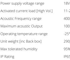
18Vdc - 40Vdc 11-25 mA at 24 Vdc 400-2900 Hz 100 dB[A]@ 1m -25° C to + 70° C 290g 95% RH [non condensing] IP65
