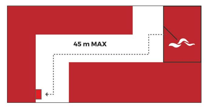
No one should have to travel more than 45m to reach the nearest Manual Call Point, or 25m in areas where a higher fire hazard is recognised, for example kitchens, paint booths etc. The 25m travel distance would also apply where a person in a wheelchair would be expected to operate a Manual Call Point.
