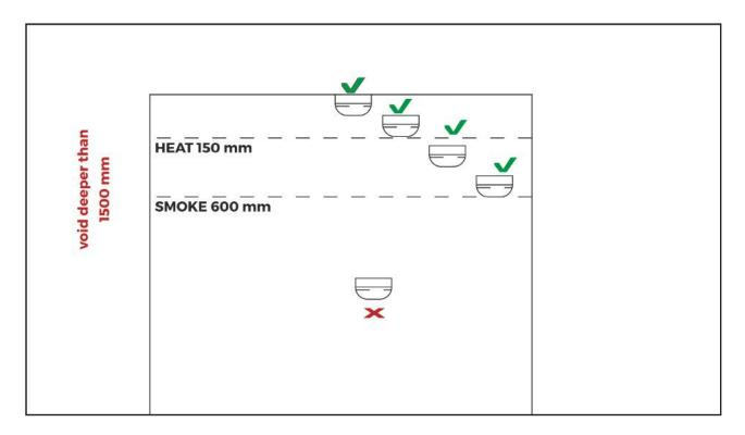
Voids deeper than 1500mm may be treated as a room when siting detectors below the ceiling - 150mm for heat and 600mm for smoke.
