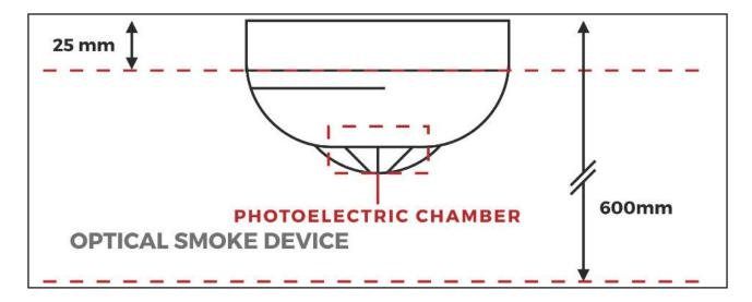
The sensing element of a Smoke detection device (photoelectric chamber) should not be less than 25mm below the ceiling, and not greater than 600mm below the ceiling.
