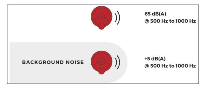
Sufficient sounders, operating within the frequency range of 500Hz to 1000Hz, should be installed to ensure that a sound pressure of 65dB(A) OR 5dB(A) above a background noise (if lasting more than 30 seconds) at all accessible points with all doors closed. This may be reduced to 60dB(A) in stairways or enclosures less than 60m² excluding corridors.
