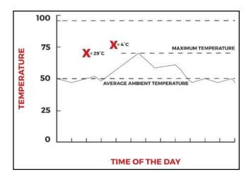
The minimum static response of heat devices should not be less than 29°C above the average ambient temperature, or less than 4°C above the highest temperature the device can be expected to experience.
