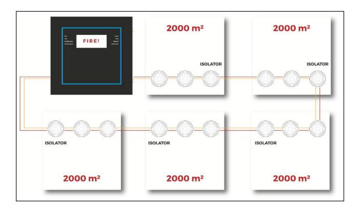
Short circuit isolators (either on the loop or within the CIE) should be installed to limit the loss of fire cover caused by a single fault to 2000m<sup>2</sup>. The loss of fire cover caused by two simultaneousn faults should be limited to 10,000m<sup>2</sup>. This will therefore restrict the cover provided by any analogue loop to 10,000m<sup>2</sup> maximum.
