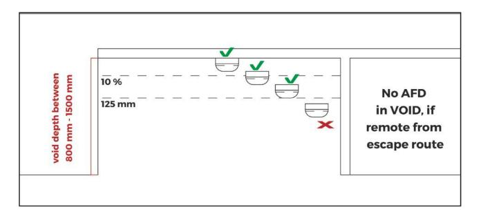
If the system category requires detection in any area, which has a void deeper than 800mm but less than 1500mm depth, detection should be provided in the void. All such detection should be sited in the top 10% or 125mm of void depth (whichever is the greater).
