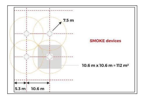
Smoke detection devices have an individual coverage of 7.5m radius. However these radii must overlap to ensure there are no "blind spots". Therefore the individual coverage can be represented by a square measuring 10.6m x 10.6m giving an area coverage of per device (usually approximated to 100m²).
