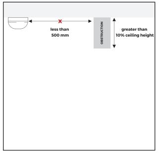
Ceiling obstructions, if deeper than 10% of the ceiling height, or floor mounted obstructions (e.g. partitions) where the top is less than 300mm from ceiling should be treated as walls. No detection device should be mounted within 500mm of any wall or obstruction treated as a wall.
