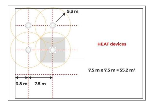
Heat detection devices have an individual coverage of 5.3m radius. However these radii must overlap to ensure there are no "blind spots". Therefore the individual coverage can be represented by a square measuring 7.5m x 7.5m giving an area coverage of 56.25m² per device (usually approximated to 50m²).
