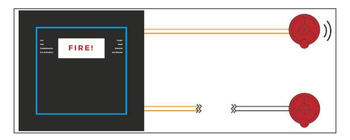
Alarm device circuits should be arranged so that, in the event of a single fault, at least one sounder, sited within the vicinity of the CIE, will continue to operate .
