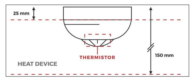
The sensing element of a Heat detection device (thermistor) should not be less than 25mm below the ceiling, and not greater than 150mm below the ceiling.
