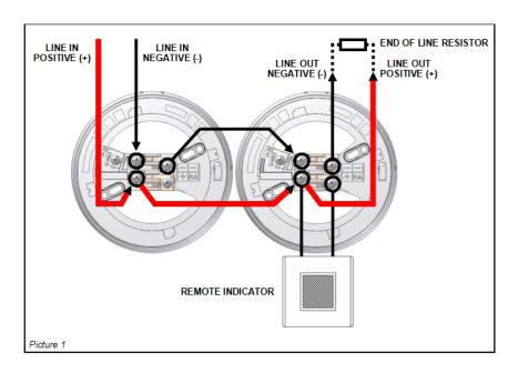
The EURVC-SD standard conventional base from the Eurotech range should be wired as shown above.
