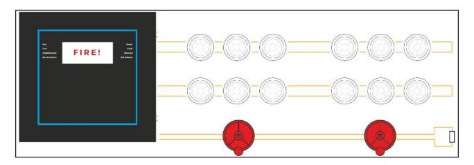
Cables used for the Critical Signal Path and the final LV (low voltage) mains supply to any fire detection equipment are now required to be fire resistant and coloured externally in a single, common colour (red is preferred). The LV supply to all parts of the system should be provided with a double pole, lockable isolation device for the safety of the maintainer. Non-critical cabling may still be non-fire resistant, for example door retainer circuitry which may fail to safe.
