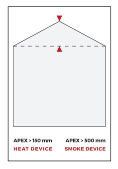
For ceilings that feature an apex: as long as the height difference between the apex and the height of the eaves is less than 150mm for Heat detectors or less than 600mm for Smoke detectors then these can be treated the same as flat ceilings. For higher apexes, a device should be installed at or near the apex. The radius of cover for this detector only may be increased by 1% for each degree of roof angle, up to a maximum of 25%.
