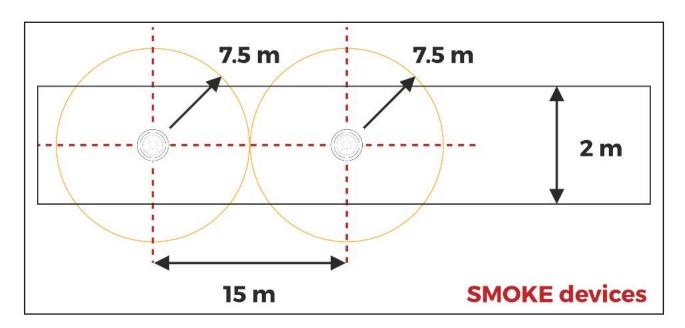
In corridors less than 2m wide the horizontal spacing of smoke detectors may be increased, the areas of coverage need not overlap as in the case of a room. Note that in corridors CO sensors can only be used in-conjunction with smoke sensors.
