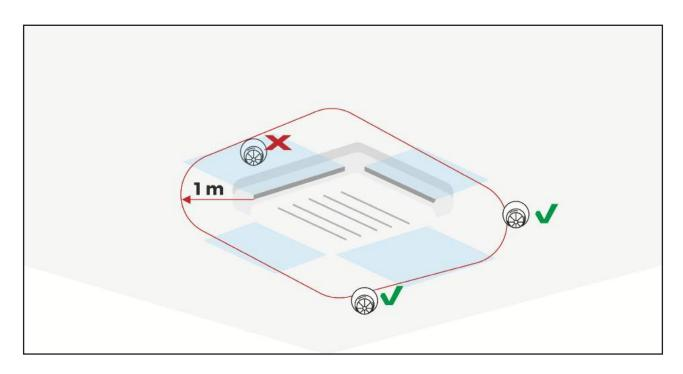
Detection devices should not be sited within 1m from air inlets or forced ventilation systems (air-conditioning).
