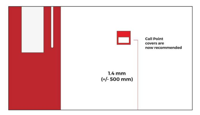
Manual Call Points should be positioned 1.4m (+/- 300mm) from finished floor level and if sited below 1.1m a variation will be required. They may be They may be semi-recessed if readily visible but if required to be seen from the side (for example, in a corridor) they should be 15mm proud of the wall.
