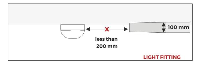
Detection devices should not be mounted closer than twice the depth of any obstruction less than 250mm and less than 10% of the ceiling height.
