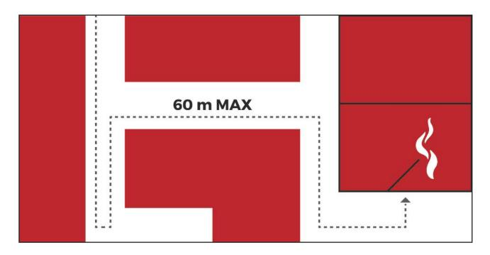
A person searching a Conventional Zone for a fire should not have to travel more than 60m from the point of entry into the Zone to identify evidence of a fire.
