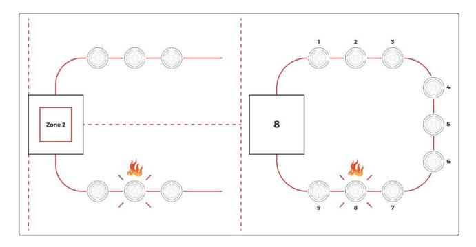
Where occupants of a building are going to need assistance from staff to evacuate the building (e.g. in residential care premises and hospitals), the fire detection and fire alarm system should be ADDRESSABLE if the building has facilities for MORE THAN 10 PEOPLE to sleep.
