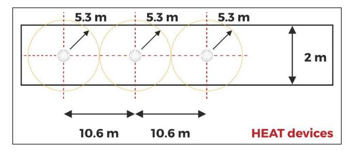
The standard does not recommend using heat sensors in escape routes, unless covered by a variation. In corridors less than 2m wide the horizontal spacing of heat detectors may be increased, the areas of coverage need not overlap as in the case of a room. If a corridor is deemed part of an escape route heat detectors should not be installed due to the possibility of smoke hazard.
