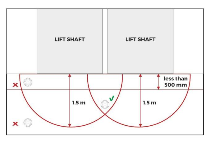
Other than in Categories L4, L5 and P2 (see page 3) any vertical flue-like structure (lift shafts, open risers etc) which penetrates one or more ceilings should have a detection device mounted at the top in the vertical structure and at each level, including the top floor, in the accommodation area, within about 1.5m of any access hatch or door opening to the vertical structure. Example lift doors are shown.
