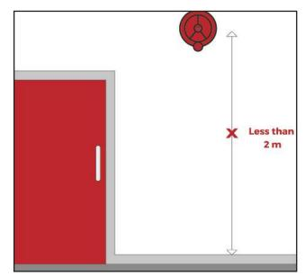
All fire alarm cables, below the height of 2m from the finished floor level should be mechanically protected, unless enhanced. If a cable passes through a floor, sleeving up to 300mm minimum should be provided. Metal fixings should be used throughout.
