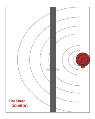
A reduction in sound pressure of approximately 20dB(A) may be expected through a normal door, and approximately 30dB(A) through a fire door.
