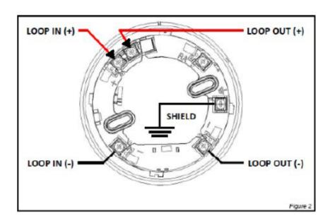
The EURB-4-EV standard analogue base from the Eurotech range should be wired as shown above. All remote indicators should be tested at least once per year and should be wired with the same grade of cable as the detection circuits (Enhanced/ Standard). This can be reduced to 1mm2 to facilitate installation.
