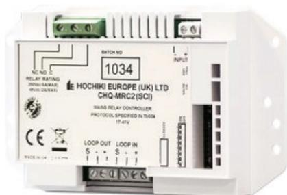
Model CHQ-MRC2(SCI) is a Single Input/Output Module, which provides a single, mains-rated relay output for the control of such devices as dampers, extractors or plant and equipment shutdown. The monitored input can be used for local power supply fault monitoring or as a general-purpose input.
